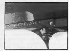
Located one on each side above the front of the trigger guard, the slide dismounting catches, when pulled downward, permit the slide group to be removed from the frame.
